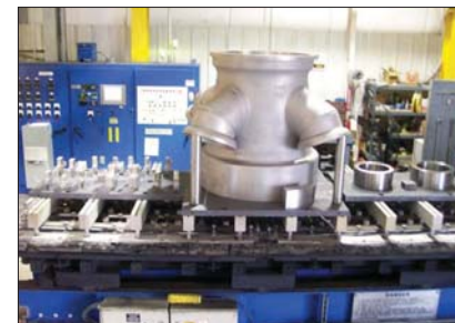
Titanium manifold weldment after vacuum heat treatment.
